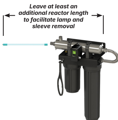
Figure 3. Lamp Removal Spacing
