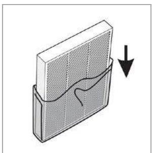
Remove any packing from the new filter element.
