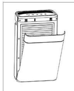
Place the new filter into the air purifier and ensure the arrow on the filter matches the direction of the flow. Refit the purifier's front cover. After replacing the filter, plug the power cord back into an electrical outlet, and hold down the filter button for 3 seconds to reset the filter timer. The indicator light will go out showing the reset was successful. (See Page 7).
