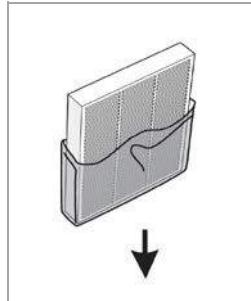
Before using the air purifier for the first time, open the front cover and remove the composite filter. Remove any packaging from the filter element to ensure the MountainAir Room will work properly. Ensure the arrow on the filter is pointing into the MountainAir Room.
