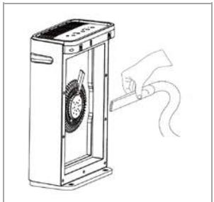
Clean out any remaining dust, dirt, or hair inside the purifier using a vacuum or dry cloth.
